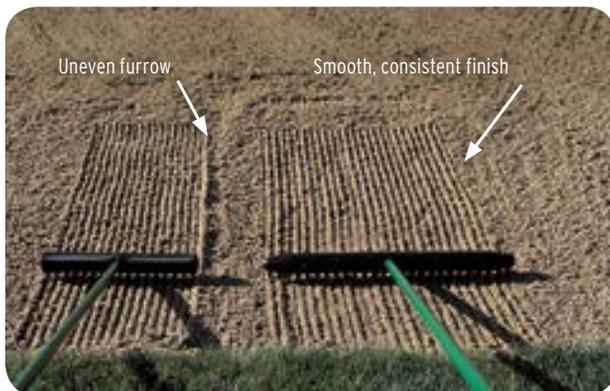
All competitive rake designs leave uneven furrows on the edges (left image). Par Aide's patented Accuform Ace II greatly reduces furrows, leaving bunkers more consistent and smooth.
