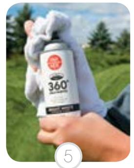
5 Place rag over nozzle and press to clear excess paint from nozzle after every 9 holes.
